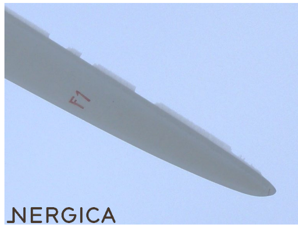
Figure 5: Example of light rime on a wind turbine blade
