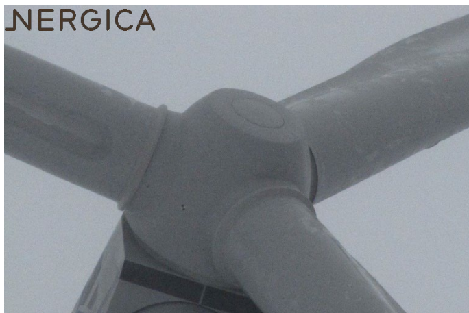
Figure 7: Typical glaze accumulation on wind turbine rotor
